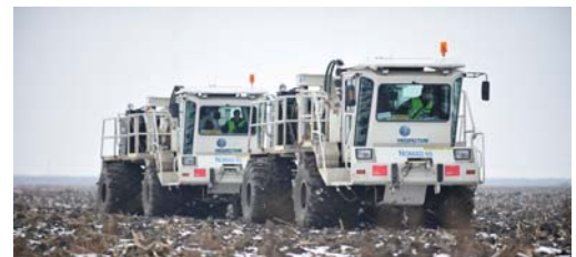
SEISMIC SURVEY: Two of Prospectiuni's specialised, vibrator trucks: These move slowly across the land, creating seismic waves which travel underground and reflect off the many subterranean rock layers. The waves bounce back to the surface and are recorded by thousands of sensitive 'geophones', which are pre-planted in the soil over large areas. Geophones are similar to microphones and are designed to detect vibration. The geophones then transmit the vibration through many kilometres of cable to a central recording truck, where our technical staff operates computers with software designed to correlate all the incoming information.
